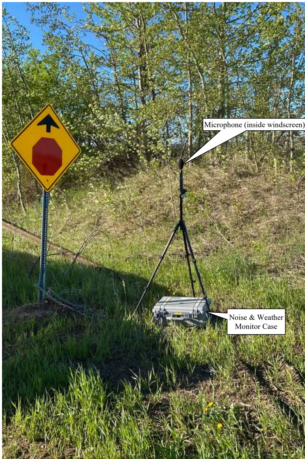
Figure 3. Example of Noise Monitor Used for Short Term Measurement
