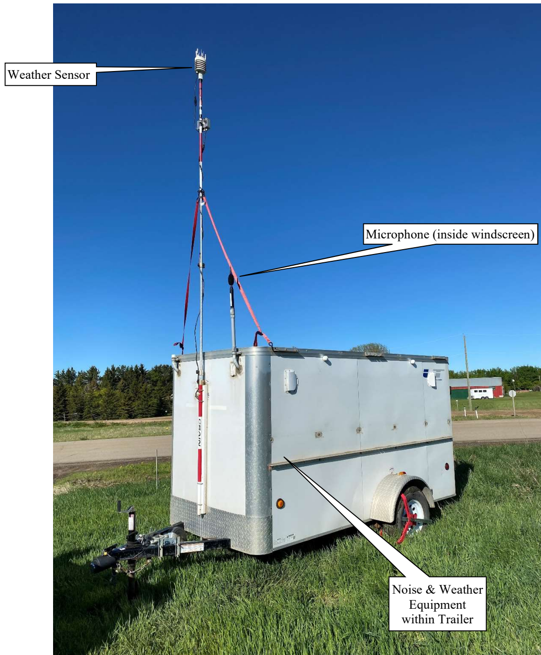
Figure 4. Noise & Weather Monitors Used for Environmental Noise Study
